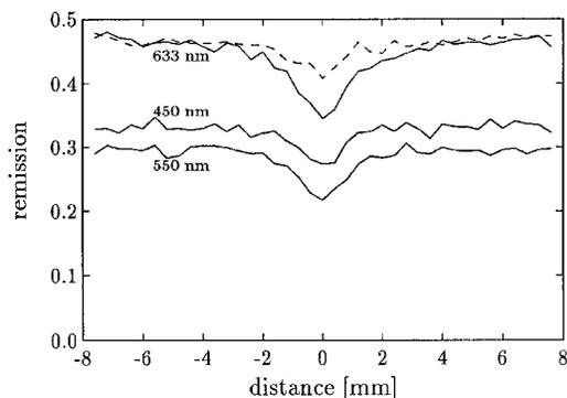
Fig. 9. Simulations of the *in vivo* vessel at 450, 550, and 633 nm. At 633 nm the dashed curve represents arterial blood and the solid curve represents venous blood. Depth  $a$  of the blood vessel is 0.5 mm, and the diameter is also 0.5 mm.
